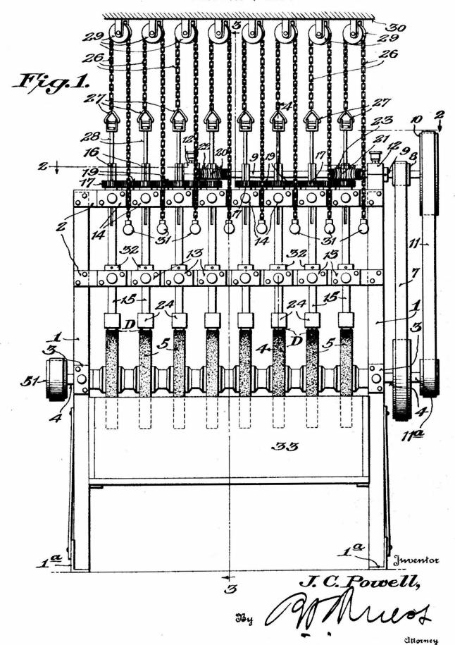
MACHINE FOR POLISHING OR GRINDING GLASS KNOBS AND SIMILAR ARTICLES
