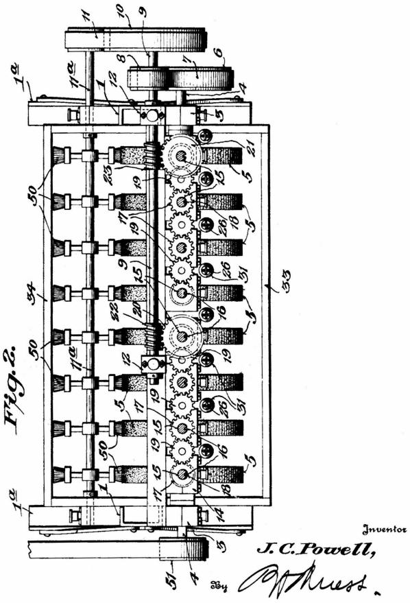
MACHINE FOR POLISHING OR GRINDING GLASS KNOBS AND SIMILAR ARTICLES
