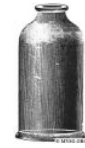
No. 632 - Bell Glass, Open Top, Ground Flange Top and Bottom All measurements are inside. Pint - 3" diameter, 6" height. Quart - 4" diameter, 8" height. (#1) 1/2 Gallon - 5" diameter, 9" height. (#2) Gallon - 6" diameter, 11" height. (#3) 2 Gallon - 7" diameter, 15" height. (#4) 3 Gallon - 8 1/2" diameter, 15" height. (#5) 5 gallon - 9 1/2" diameter, 18" height.
