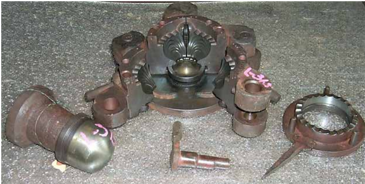
A press mould from The Cambridge Glass Company had five different parts: base, shell, plunger, ring and key. This mould is from the popular Cambridge Caprice line! Any guess on how much this weighs?
