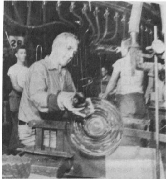
A piece of wood is used to shape the glass
