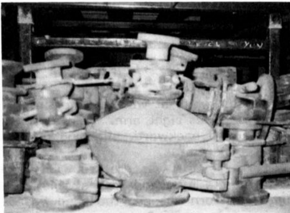
Pallet containing a mixture of both PASTE (Blow) and IRON (Press) Molds
